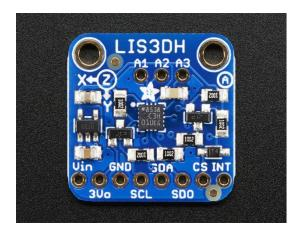
The accelerometer sensor I researched is the Adafruit LIS3DH, I picked this sensor because it had the lowest power draw of the sensors that I looked at. The power draw is only 2uA which is good because part of the project is to try and the power draw as low as possible. I choose to research an accelerometer sensor as I thought this would be the sensor that would most fit the project as it can detect any movements of the lifebuoy.
