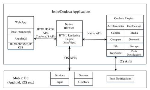
Figure 9. IONIC Architecture [Qian16]
