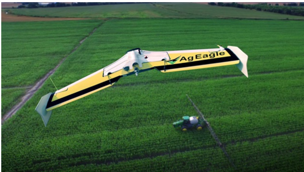
Figure 1: Fixed-wing AgEagle EX-60 Drone. Source: ageagle.com
